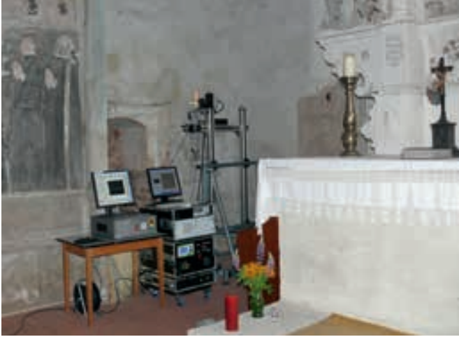
THz measurements of actual hidden wall paintings, here at the church in Beesdau (Brandenburg)
